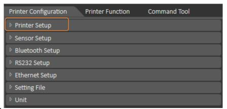
2. Click the Load Button to bring out all printer general setting information through the selected communication interface. Click the Set button to write the setting value to the printer (please execute the reading function before writing).
