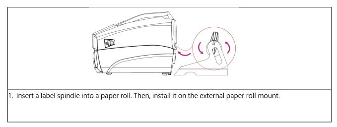
Note: When using the Gainscha External Label holder, the 1" core label spindle only supports a radius of 12 cm / 2" core label spindle only supports a radius of 10 cm / 3" core label spindle only supports a radius of 8.5 cm
