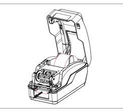
Pull out the print media till it pass sensor; adjust the paper guide to be same width of print media, complete media loading.
