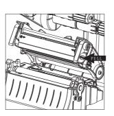
3. Pull the Print head release lever to open
