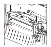
6. Close the print head mechanism on both sides and make sure the latches are engaged securely. Set media sensor type and calibrate the selected sensor
