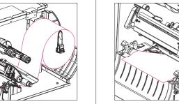
4. Install the label through the media guide bar, damper, media sensor, and label guide to install 5. Move the media sensor by adjusting the media sensor position adjustment knob, make sure the the media. (See the "Media Loading Path" gap or black mark sensor is at the location where media gap/black mark will pass through for sensing Adjust the label guide to fix the media position. illustration below).
