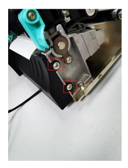
2. Remove the sensor and baffle screws.
