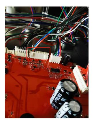
**8.** The blue cable end of the cutter main board is inserted into the "No.1" interface just removed in the figure below:
