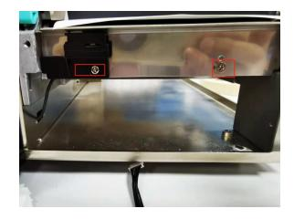
**3.** Remove the side housing screws of the printer.
