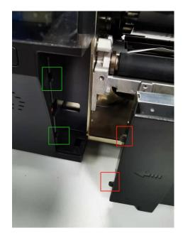
**14.**The two screws for mounting the cutter are shown below:
