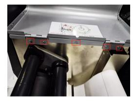
**5.** Remove the side baffle and hood of the printer.
