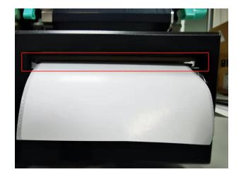
**16.**Check whether the cutter is successfully installed, the printer is powered on, open the printer switch, and click on the upper left corner in the figure below:
