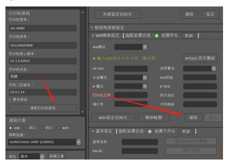
3. After reading, the AP name, IP address, and port number indicate the success of installing the WiFi module in the following figure:
