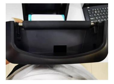
3. Open the two bars under the rubber stick first inside and then up.
