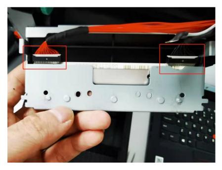
**7.** Install the print head : put the print head in the thermal bracket, pay attention to the front and back of the print head, and connect the print head online:
