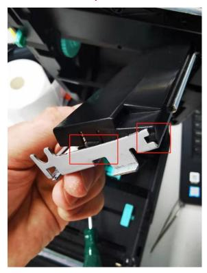
9.Install two fixed screws on the print head (note: the right screw must be plugged with a white coil gasket):
