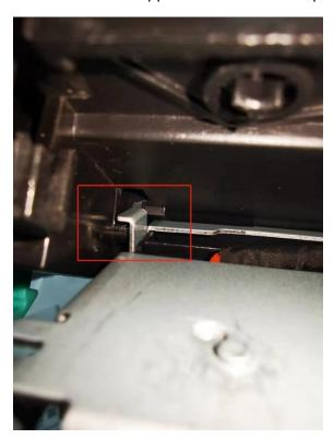
**11.**The bumps on the bracket must be stuck in place:
