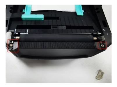
2. Lift the baffle up and remove the baffle.
