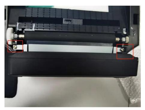
**11.**The label passes through the cutter interior as shown below.
