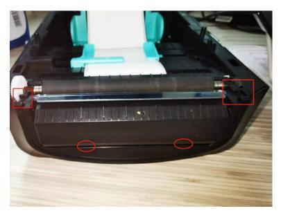
10. Open the stripper and pass the label bottom paper through the stripper as shown in the figure below:
