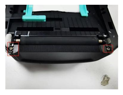
2. Lift the baffle up, and remove it:
