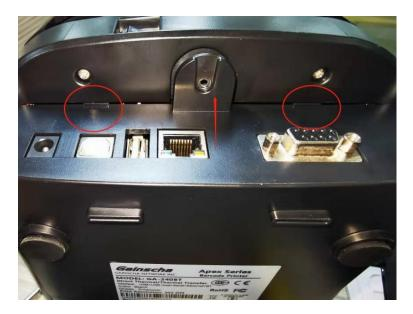
8. Card the bump of the stripper into the groove as shown below:
