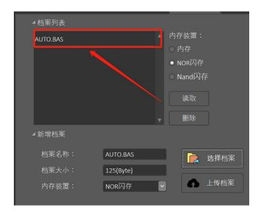
**8.** Restart the printer and read the file list; the file name is uploaded successfully
