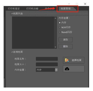
**4.** Select NOR Flash or Nand Flash Note: (NOR flash is a random storage medium for small data volume; NAND flash is a continuous storage medium, suitable for large data, please select according to the data size.)
